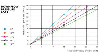
Bed expansion and pressure loss curves are provided for the most commonly used particle sizes. Charts are available for all particle sizes on request.
