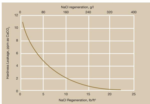
Capacity and Hardness Leakage graphs are shown assuming a service flow of 4 gpm/ft<sup>2</sup> (32 l/h/m<sup>2</sup>) and total dissolved solids of 400 ppm and 20 grains of total hardness. The hardness leakage will increase and the capacity will decrease while increasing total dissolved solids and total hardness.
