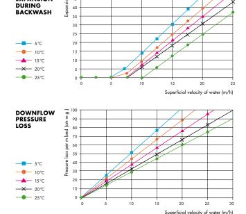
Bed expansion and pressure loss curves are provided for the most commonly used particle sizes. Charts are available for all particle sizes on request.
